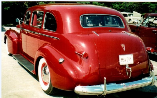
1940 Cadillac with integrated trunk and exposed gas cap
