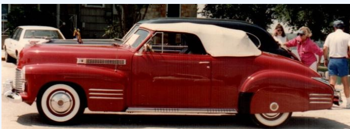
1941 Cadillac convertible - first year. Egg crate grill, outboard mounted head lamps, hydraulic lifters, 346 cu. in. V-8, anti roll bars, center panel AM radio, gas filler cap under left taillight, optional fog lamps, back-up lights, vacuum aerials, air conditioning, and hydramatic drive - standard on 1950 62 series!
